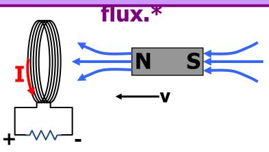
If Lenz's law were not true—if there were a + sign in Faraday's law—then a changing magnetic field would produce a current, which would further increase the magnetic field, further increasing the current, making the magnetic field still bigger...
