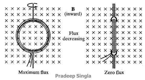
Example: a uniform (but time-varying) magnetic field passes through a circular coil whose normal is parallel to the magnetic field. The coil's area is  $10^{-2}$  m<sup>2</sup> and it has a resistance of 1 m $\Omega$ . B varies with time as shown in the graph. Plot the current in the coil
