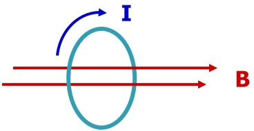
A constant magnetic flux does not induce an emf—it takes a changing magnetic flux.
