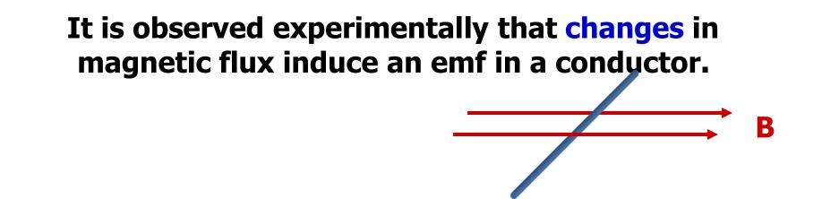
An electric current is induced if there is a closed circuit (e.g., loop of wire) in the changing magnetic flux.
