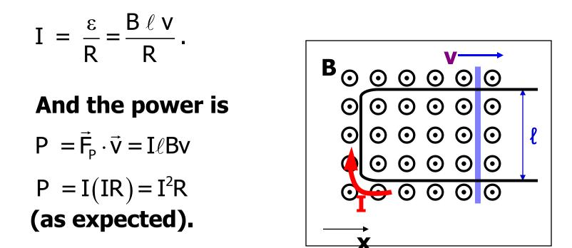
Mechanical energy (from the pulling force) has been converted into electrical energy, and the electrical energy is then dissipated by the resistance of the wire.
